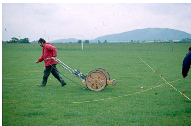
Figure 1.14: Novel caesium vapour magnetometers at Wroxeter: left Joerg Fassbinder, right, Archaeophysica. (Photos R White)
