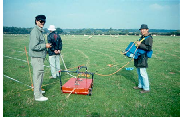
Figure 1.32: Dean Goodman (l) and Yasushi Nishimura (r) undertaking a GPR survey at Wroxeter, 1998. (Photo R. White)
