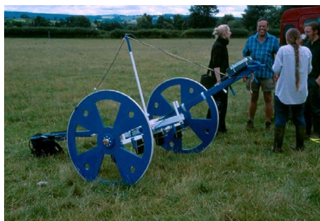
Figure 1.14: Novel caesium vapour magnetometers at Wroxeter: left Joerg Fassbinder, right, Archaeophysica. (Photos R White)
