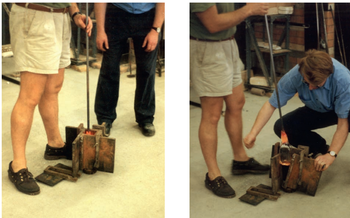
Figure 1.3. Bill Gudenrath demonstrating how to blow a square bottle in a five-piece mould at the Glass Techniques through 5000 Years conference held at the Edinburgh College of Art, 24-27 September 1992. On the left the bottle being inflated in the mould. On the right Ray Flavel, acting as the assistant, is rapidly dismantling the pieces at the end of the process.
