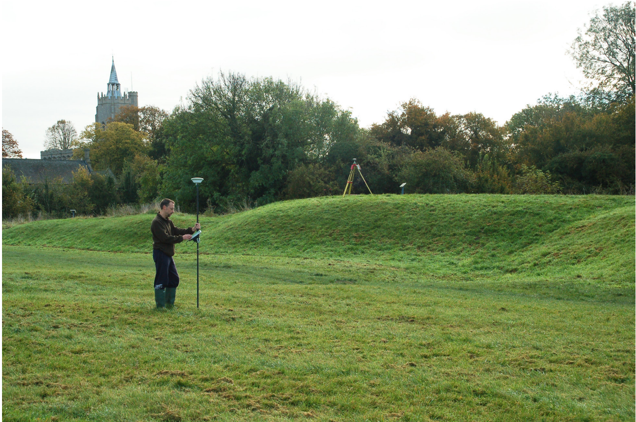
FIGURE 1.3: TOPOGRAPHICAL SURVEY USING DIFFERENTIAL GPS AT BURWELL CASTLE, CAMBRIDGESHIRE, FOR THE WAR AND STATUS PROJECT. THE EARTHWORKS IN THE BACKGROUND ARE HEAPS OF SPOIL CREATED DURING THE CONSTRUCTION OF THE MOAT OF AN UNFINISHED ROYAL CAMPAIGN CASTLE BUILT FOR KING STEPHEN ON THE FEN EDGE (THIS VOLUME, CHAPTER 2 FOR DISCUSSION).
