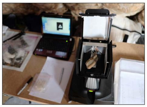
Fig. 1.17 Archaeological ceramic sherd being non-invasively geochemically characterised via portable X-ray fluorescence spectroscopy (pXRF). The sherd has been placed within a lead-lined chamber (open for illustrative purposes) over the beam and detector of the instrument, and data is being recorded on a laptop. Roman pottery, England.
