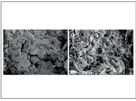
Fig. 1.15 Clay vitrification microstructure of archaeological ceramic sherds in the SEM. The sample on the left exhibits a rough appearance from the presence of the clay minerals, whereas on the right these have vitrified to form a glassy network. Neolithic pottery, Serbia. Image width = 0.1 mm (L) and 0.05 mm (R). Modified from Amicone et al. (2020, fig. 6).
