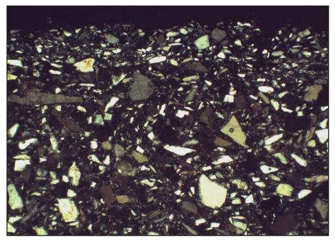
Fig. 1.23 Fritware/stonepaste ceramic artefact in thin section composed of angular, crushed quartz inclusions set in a glassy, isotropic matrix with abundant voids. The sample has a fritted glaze applied to the exterior. Islamic pottery, Turkmenistan. XP. Image width =2.9 mm.
