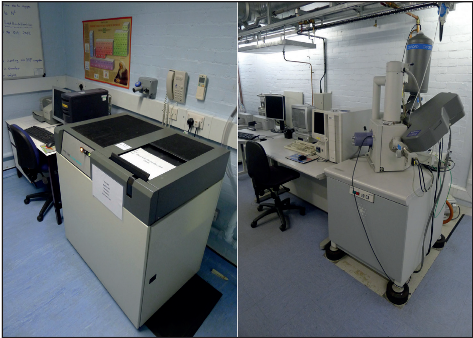
Fig. 1.3 Apparatus used for the instrumental analysis of archaeological ceramics. An X-ray fluorescence spectrometer (XRF) (left) and a scanning electron microscope with an energy-dispersive spectrometer (SEM-EDS) (right).
