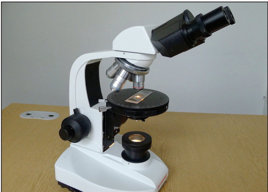
Fig. 1.4 A simple, inexpensive polarizing light microscope being used to examine an archaeological ceramic thin section. Detailed compositional analysis can be performed on such a microscope, which has several objectives, an analyser and a graticule.
