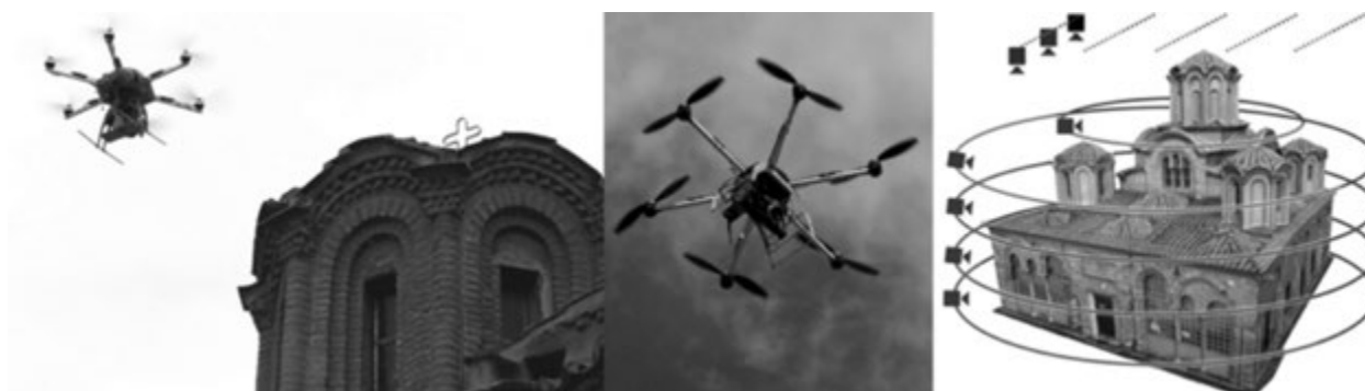
FIG. 3. UAV-BASED AERIAL DATA COLLECTION AND ILLUSTRATION OF THE MULTIPLE CLOSED LOOP PHOTO SHOOTING APPROACH.
