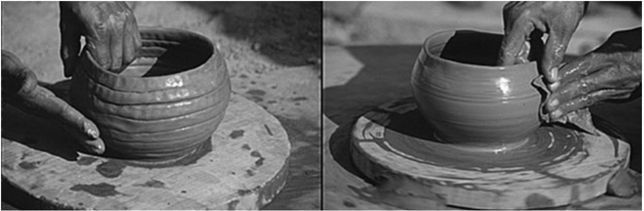
FIG. 2. WHEEL COILING TECHNIQUE: ROUGH-OUT MADE OF ASSEMBLED COILS AND THEN SHAPED AND THINNED WITH ROTATIVE KINETIC ENERGY (AFTER BOILEAU 2009).
