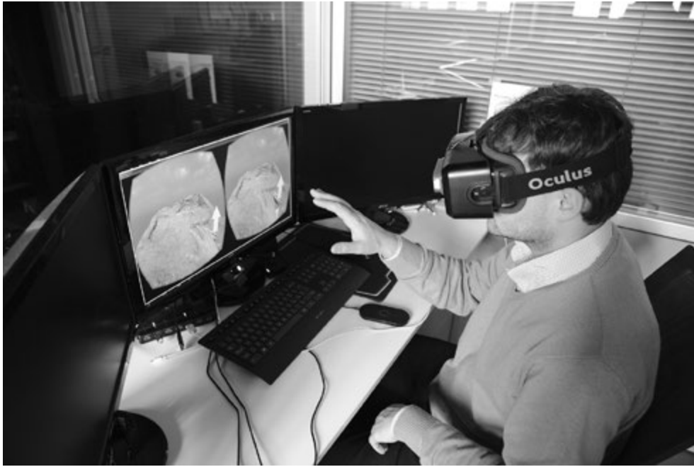
FIG. 7. THE APPLICATION COMBINING THE OCULUS RIFT DK2 AND THE LEAP SENSOR.
