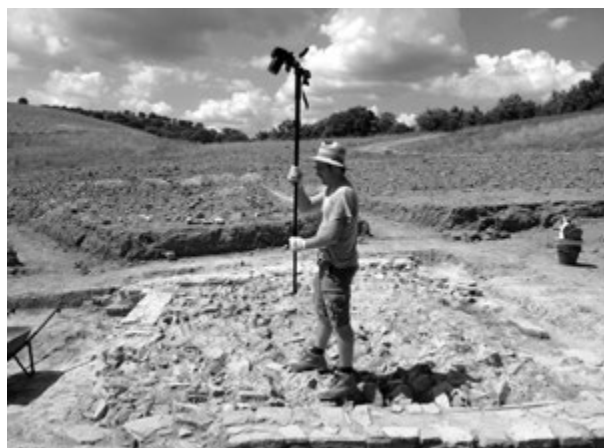
FIG. 2. MONOPOD USED IN TERRESTRIAL IMAGE ACQUISITION.
