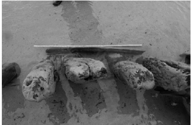
Figure 32. Frames (first futtocks) 16cm moulded 11.5cm sided and length unknown.
