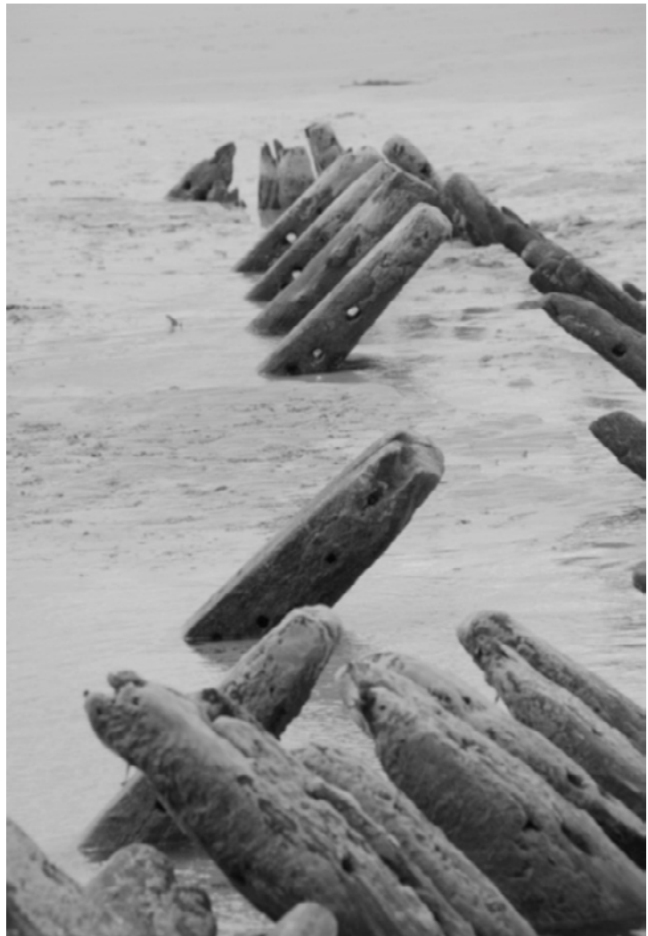
Figure 33. Image showing longitudinally aligned circular holes running through the lower deck beams
