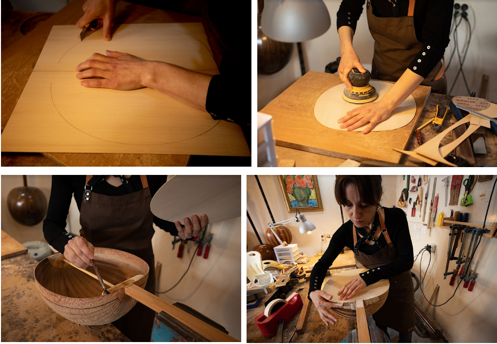
Figure 45. Processing of the ultra-thin two-piece soundboard. © Courtesy Elif Kızılhan, Kadıköy, İstanbul.
