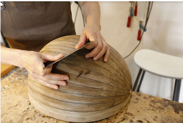
Figure 43. The ribs are attached to each other over a mold using a heating machine or a heated tool after which the bowl is finished. © Courtesy Elif Kızılhan, Kadıköy, Istanbul.
