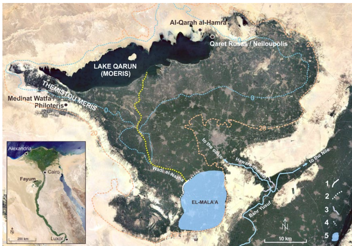
Figure 1. Satellite image of the Fayum Oasis (Google). 1 – section of the dam forming the el-Mala'a basin; 2 – reconstructed sections of the dam forming the el-Mala'a basin; 3 – partly preserved sections of the dams at the entrance to the Hawara channel; 4 – reconstructed sections of the dam at the entrance to the Hawara channel; 5 – hypothetical extent of el-Mala'a basin. Contour lines 0 and 20 ASL after Hassan 1986: 484, fig. 1; location of dams forming the el-Mala'a basin and near the entrance to the Hawara channel, and the extent of el-Mala'a basin after Garbrecht 1996: figs 4, 5 and 15; location of Wadi el-Nazha after Bagnall and Rathbone 2004: 128, fig. 5.1.1.
