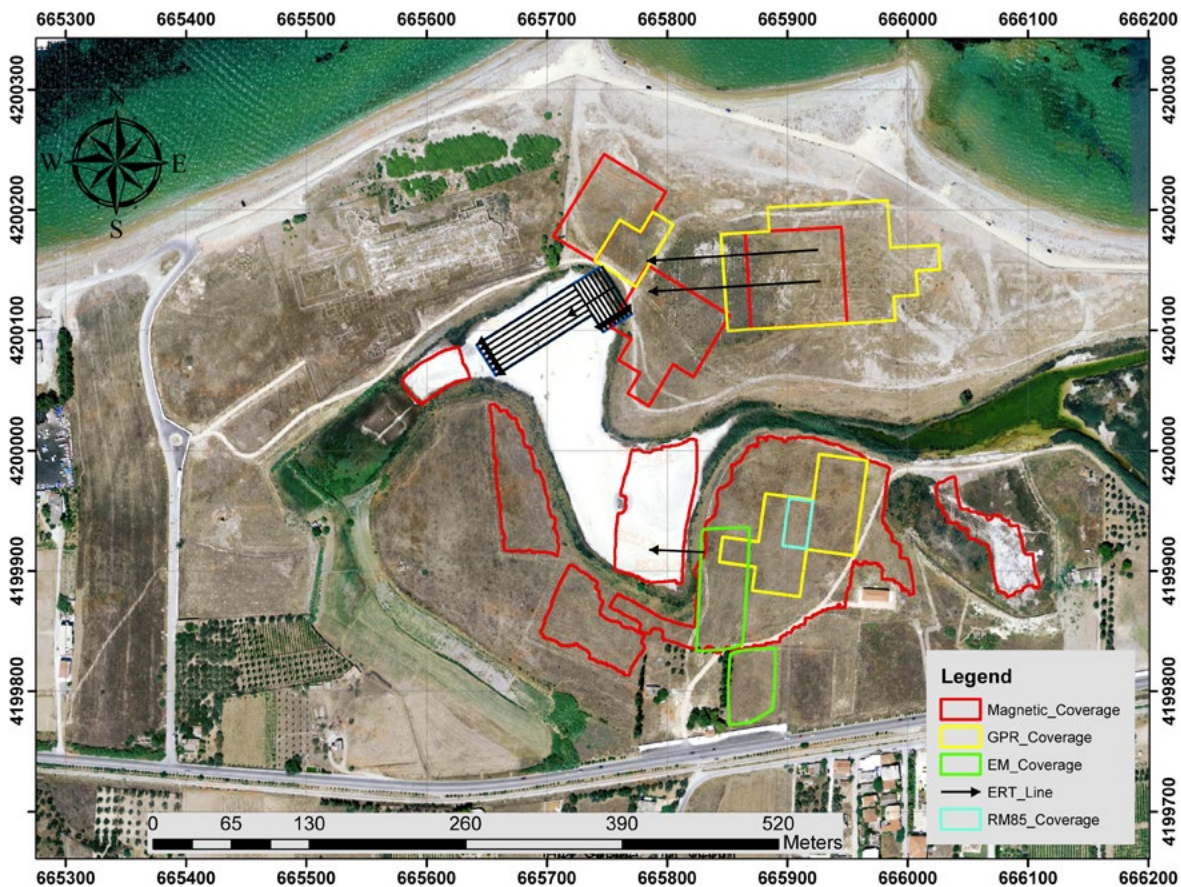
Figure 1. Area coverage from the various geophysical survey techniques during the first two fieldwork campaigns at Lechaion, Peloponnese.
