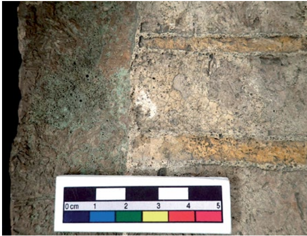
Figure 8. Tile N2067 with partly better-preserved areas of glaze showing a smooth surface and fewer bubbles. Compare with Figure 3b for location (Manuela Lehmann).
