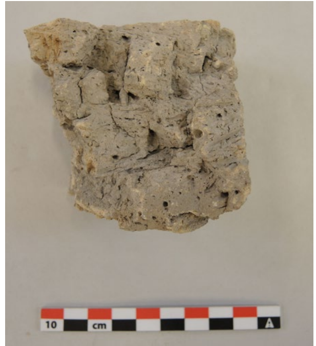
Figure 16. Brick with traces of plant-based additive (© A. Thomas 2019).
